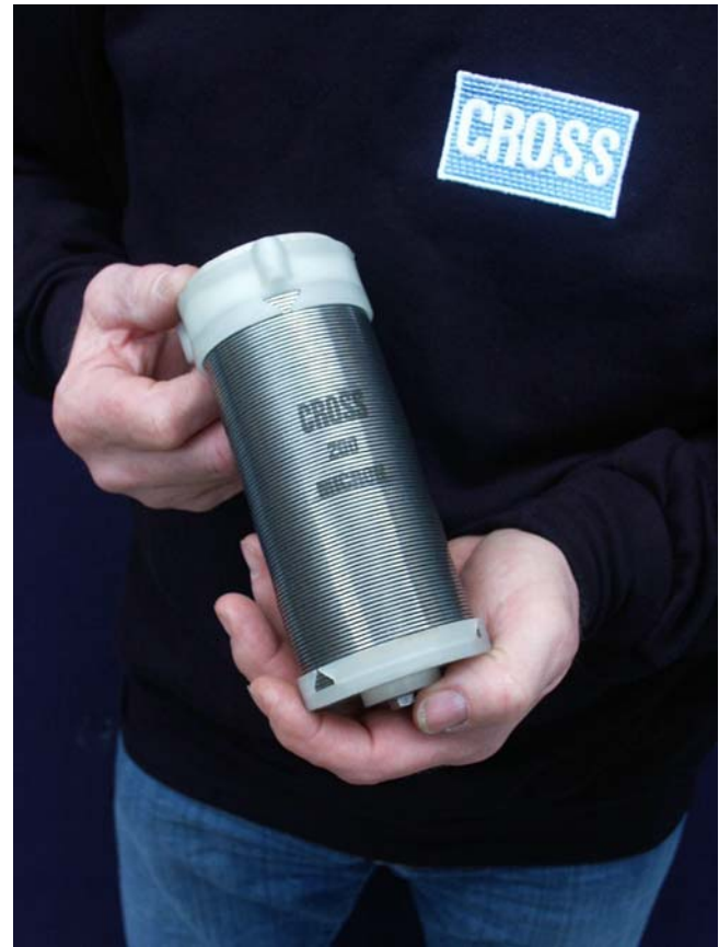
The “zero-gravity” coil that is central to Cross filtration technology. In this example, any particle larger than 200 microns is unable to pass between the coils, which open evenly along their entire length during backwashing to completely remove the build-up of debris.
