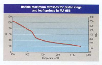
Tests at Cross showed that MA 956 piston rings consistently retained their springiness at extreme temperatures
