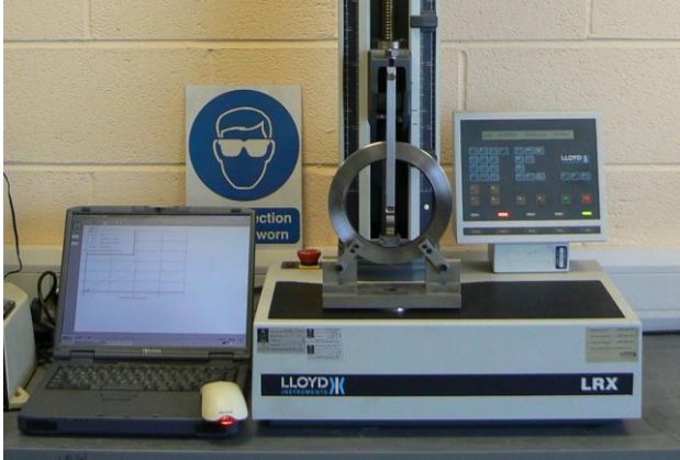
Figure 20 Stiffness Checking Machine
